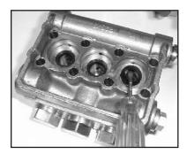
7) Remove the pressure rings (24), and v-sleeves (23) and spacer ring (23A) from the valve casing (26). Remove the remaining v-sleeves (23B) and pressure rings (24) from the seal case (20).
